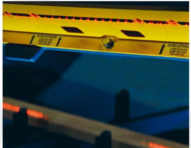
The cameras use dot lasers as well as tracheid and vision technique. The laser light is spread differently depending on the properties of the wood. This information makes it possible to better detect defects when combining it with colour and profiling measurement. One example is the detection of bright knots.
